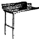
DISHTABLE, CLEAN<br>CMA Dishmachines Model No CL-60<br>Clean Dishtable, 60" long, straight design, on machine left, right to left operation, 9" high splash, galvanized steel legs, with adjustable side crossrails, 16/304 s/s                                               | 478 75    | 478 75     |
